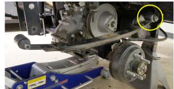
7. Orient the riser block so the leg with the hole faces the front of the cart. Place the riser block between the axle and the leaf spring. The forward facing hole will line up with the alignment pin on the axle.
